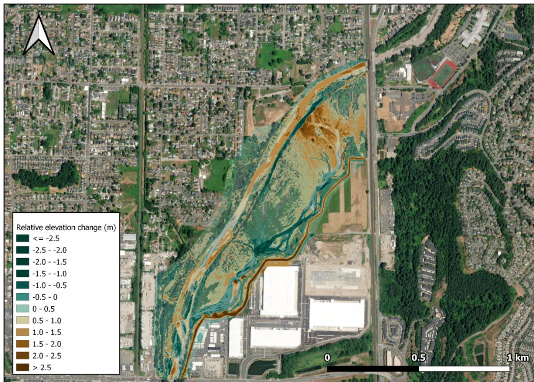
Figure 16. Relative elevation change at Countyline from 2011 to 2022 based on topo-bathymetric LiDAR.
