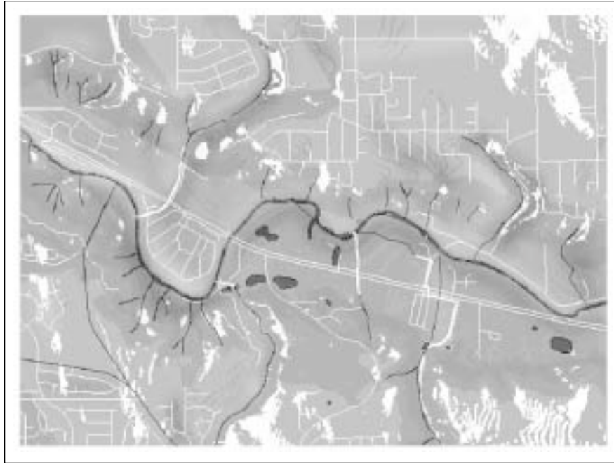
Figure 18. Depiction of loss of lateral connectivity within the floodplain. Shows diking of the mainstem, ditching of tributaries, and constructing of roads.
